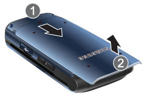
To remove the battery, pull the top of the battery away from the phone (1) and disconnect it (2).
