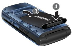
3. To replace the cover plate, slide it toward the handset (1) and push on the thumb tab (2).
